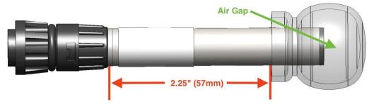
Do not handle or remove a wet windscreen as it is easy to accidentally squeeze the windscreen and push water into the end of the mic
