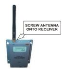
The receiver can be mounted vertically using the screw holes provided, or rested in a hori-
