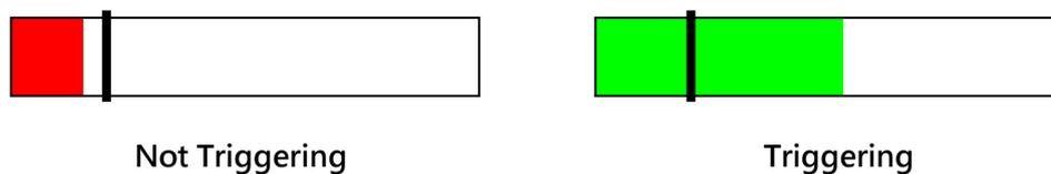
To change the sensitivity, tap on the **VU Meter** where the trigger point should be (left to increase, right to decrease sensitivity), or press the arrows on either side of the **Sensitivity** number. A higher number is more sensitive. A typical sensitivity value is 16. It should be noted that the noise level when deploying may be different to when you are recording and this should be kept in mind when setting the sensitivity.
