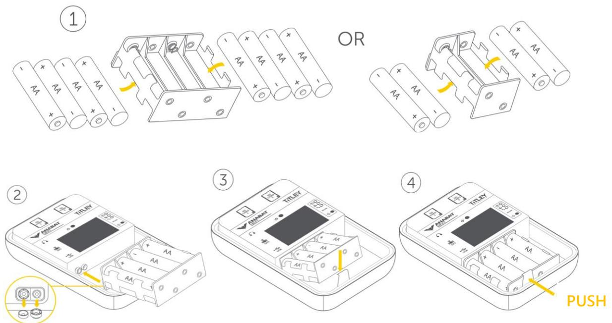
**IMPORTANT:** Do not allow the battery holder terminals to short out against metal objects. Always remove the batteries from the holder as soon as it is disconnected from the Swift. Do not store batteries in the holder.
