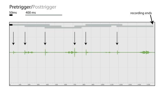
The graph explains pre- and posttrigger times of the *batcorder*. Arrows indicate positive trigger events (= bat calls). The pretrigger of 50 ms is not adjustable.
