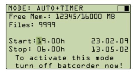
To activate this mode, switch to the display shown above via the **MODE** key (MODE: AUTO+TIMER)
