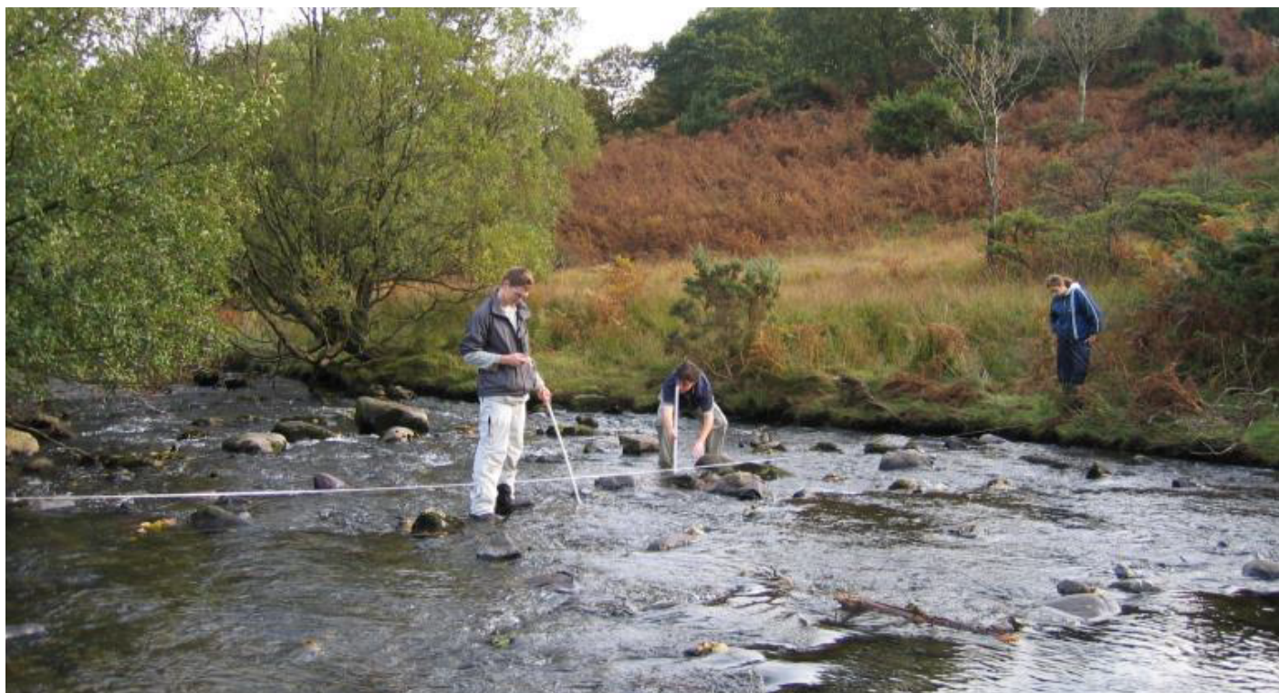
Figure 7 - Measuring "Distance Out" using tape secured at each end
