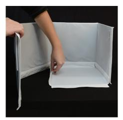
**1.** Assemble the trap container by attaching the walls and base together using the Velcro strips.
