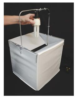
**6.** Screw in the blacklight bulb tightly to ensure a waterproof seal.
