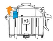
This camera can also be powered by an external 12-volt DC input such as a 12-volt battery (KIT-12V, BATT-12V or KIT6V/12V) or a 12-volt adapter (AD-12V), sold separately.
